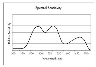
HARMAN GDS FB paper exposed for 10<sup>4</sup> seconds to broad-band colour filters illuminated by a xenon flash tube. Developer: MULTIGRADE diluted 1+9. Development: 1 minute at 20°C/68°F.
